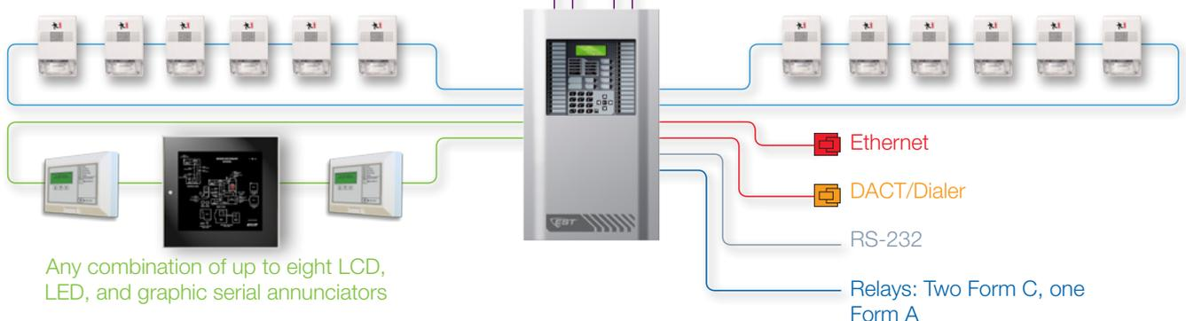
*Diagram represents an iO500 system wired for Class A operation with a full complement of option cards.*
